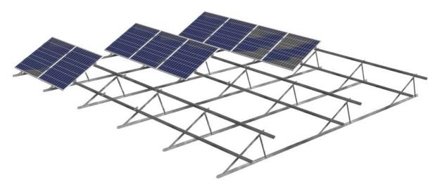
**Profi Kompakt** is a modification of the well-tried **flat roof support Schletter Profi**. If the erection can not be fastened to vertical rafters (e.g. eternit or trapezoidal sheet metal roof with transverse purlins) a vertical bridging is necessary. **Profi Kompakt** uses the vertical rail at the same time as bridging and base of the module erection and thus **saves material and mounting time!**
